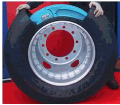
Figure 2. Military Run-flat Tire with Insert [1]
