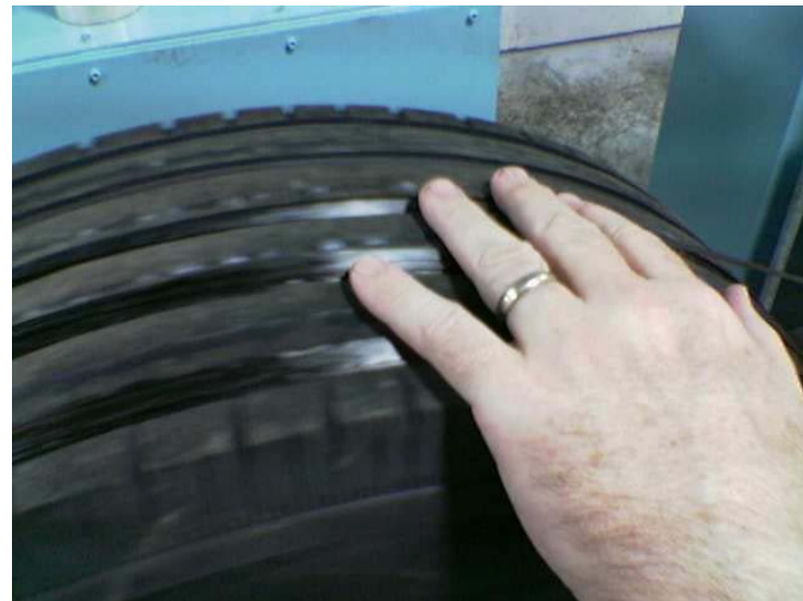
Figure 8. In Process Prototype Carbon Fiber Hoop Ring Molded Tire
